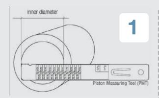
Use the Piston Measurement Tool (PMT) to measure the inner diameter of the piston. Simple and accurate.
