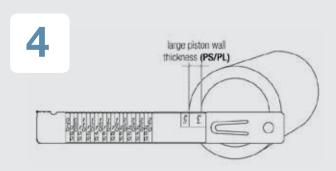
Determine the piston wall thickness and combine it with the piston diameter to find the right Piston Cushion from your Kit.
