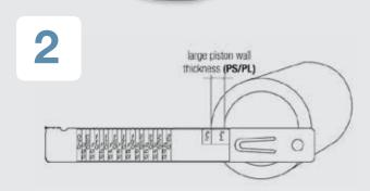
Determine the piston wall thickness and combine it with the piston diameter to find the right Piston Cushion from your Kit.
