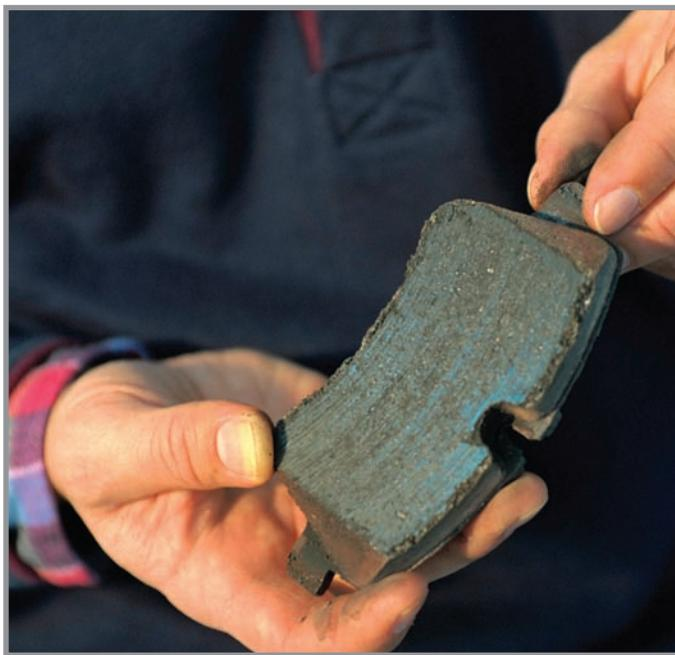
*Friction material must be able to maintain a firm hold on the backing plate under high shear loads and extreme heat, while being placed in a corrosive environment for an extended amount of time.*
