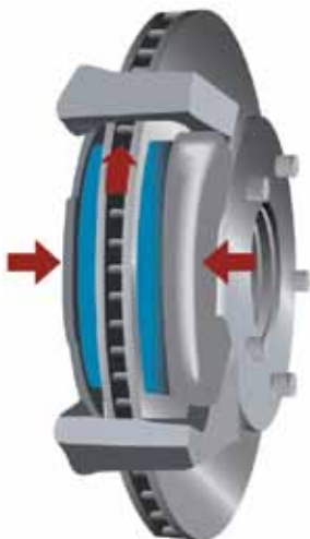
"Finger" torques under load, allowing plate to move during braking without stressing shim material or attachment
