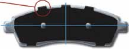
NU-LOK "fingers" under tension in locked position
